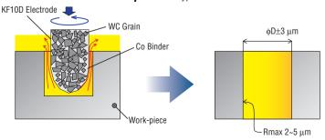
[Schematic Drawing of Electrical Discharge Process]
